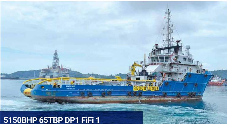
5150BHP 65TBP DP1 FiFi 1 Anchor Handling Tug Supply Standby Escort & Rescue Tug
