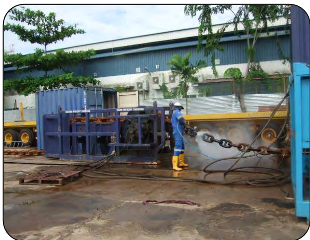
Refurbishment, Maintenance and Hydro-Jetting of Anchor Chain
