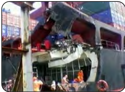
Degree of Wreckage after its collision with a VLCC Tanker along Malacca Straits
