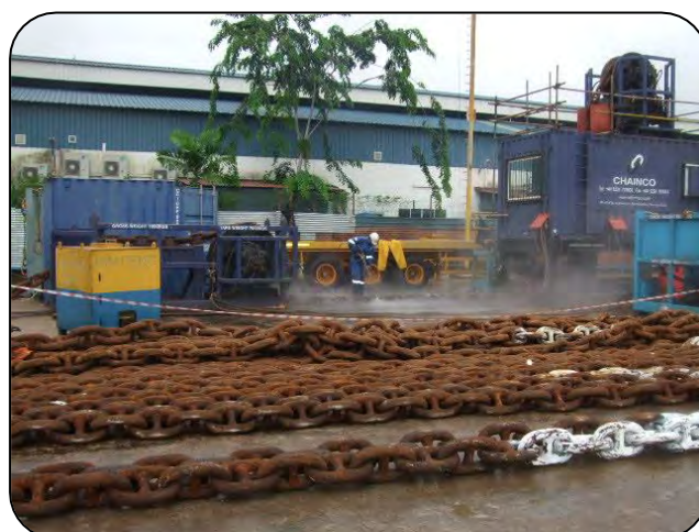
Refurbishment, Maintenance and Hydro-Jetting of Anchor Chain
