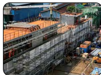
Erection & Installation of Accommodation onto Main Deck
