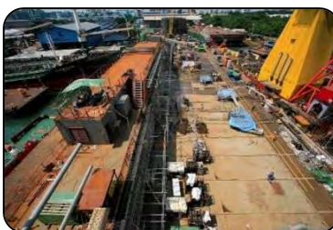
Erection & Installation of Accommodation onto Main Deck
