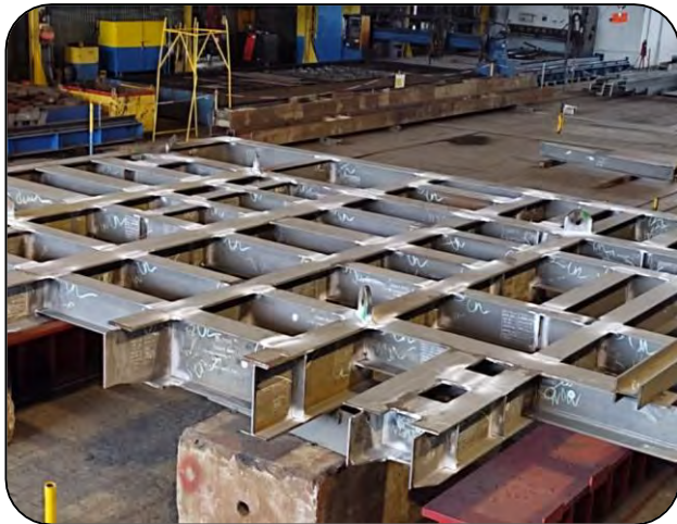
Fabrication of superstructure in segments
